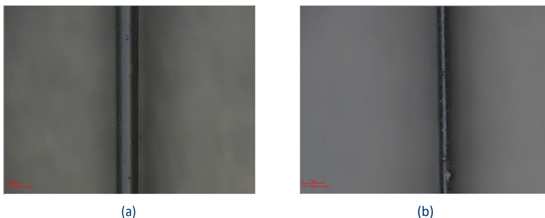
Figure 14. Melt spun precursor fibre using (a) refined asphaltene (28.38 \mu\text{m} ) and (b) polymer/additive blended asphaltene (8.90 \mu\text{m} ).
