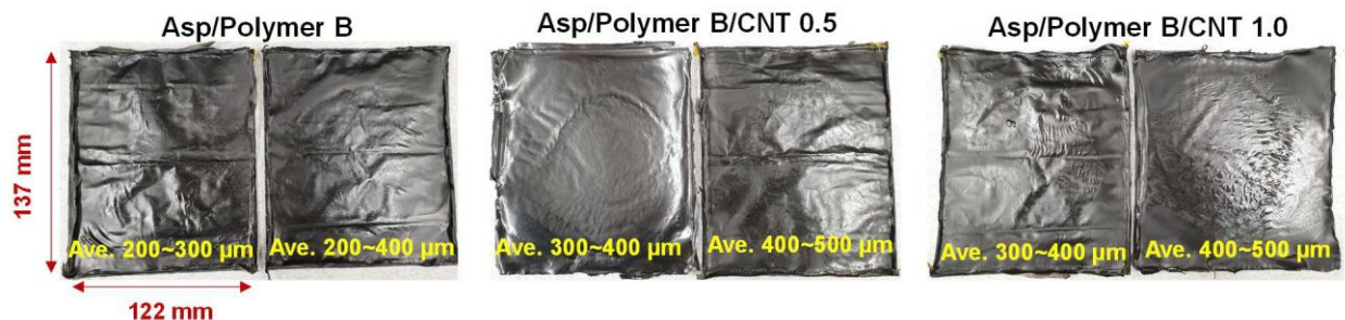
Figure 13. Pictures and thickness of Polymer B/CNT blending asphaltene films.
