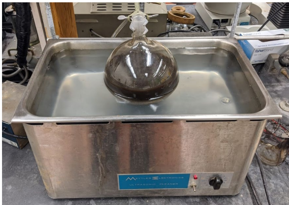
Figure 3: Sonication of toluene soluble residue and C5 mixture to precipitate C5 asphaltenes
