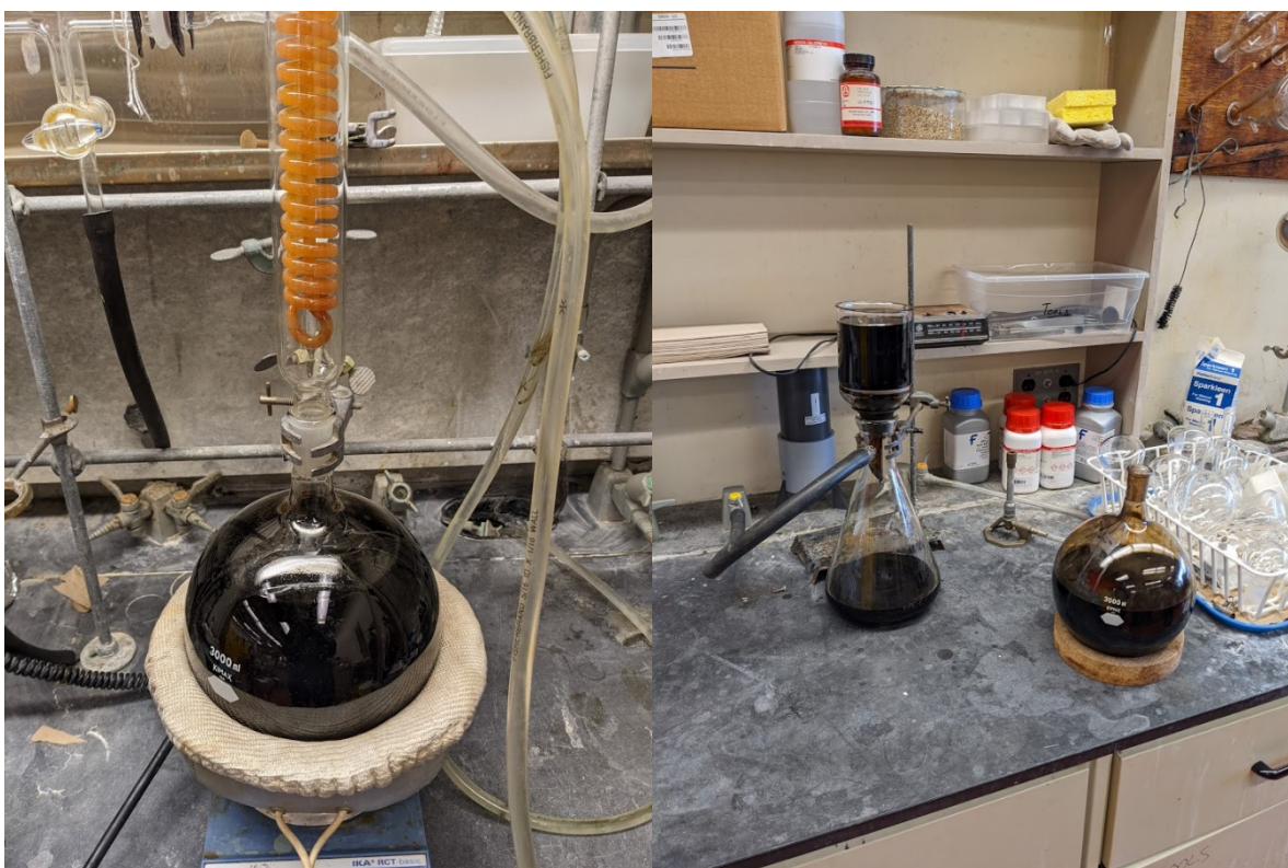
Figure 2: The asphaltene extraction procedure showing the heating and filtering steps, respectively.
