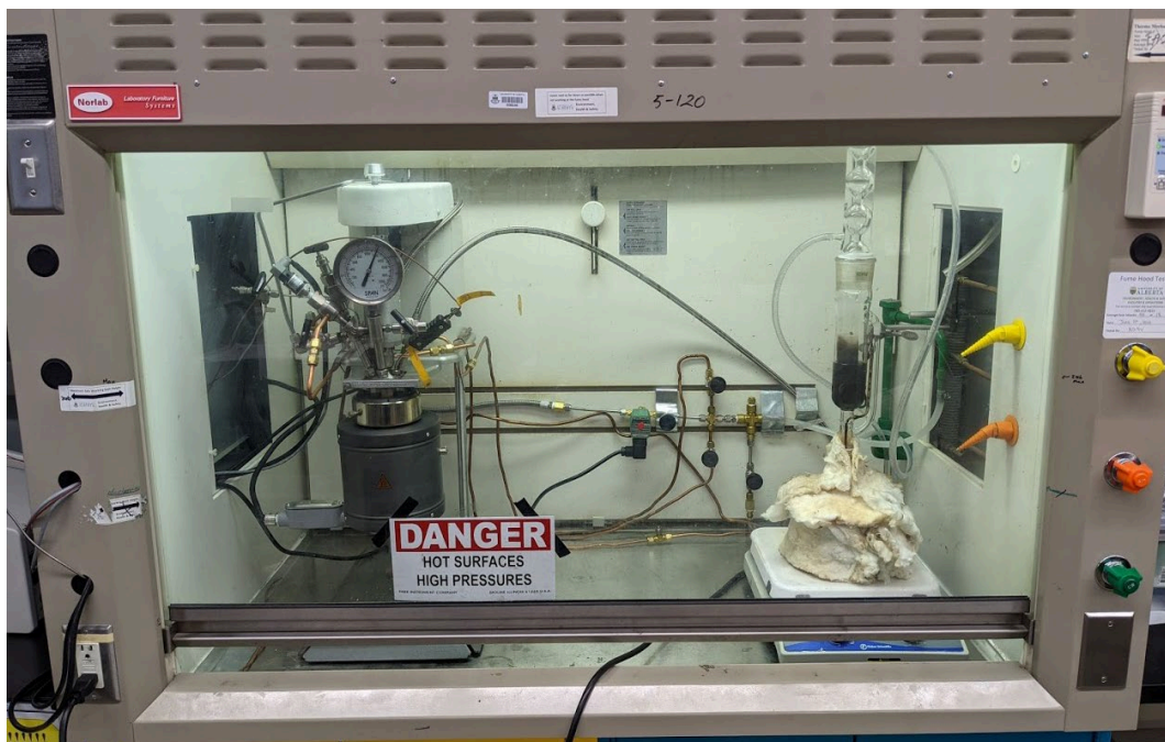
Figure 5: (Right) Parr Instruments reactor installed under fume hood where the pyrolysis took place and. (Left) Recovery of toluene from dissolved asphaltenes.
