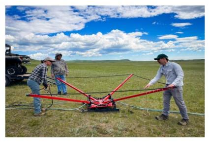
Preparing the towed time-domain-electromagnetic (tTEM) system for use to locate, map and characterize shallow groundwater resources, providing important data for water resource management.
