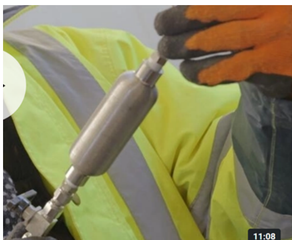
Figure 15: The downhole SysMoG™ probe
