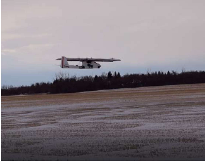
Figure 7. Small RPAS unit carrying A3S software package in fuselage over farmers field with small layer of snow on ground. Aircraft ready to perform avoidance maneuvers once Drone Configured Command Line Interface sends simulated contact to A3S.
